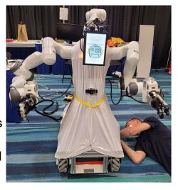
The avatar robot has five-finger hands, and its head is mounted on a robotic arm to increase its range of motion. An operator uses a VR headset with two robotic arms and hand exoskeletons, which measure the operator's arm and finger movements and provide force and haptic feedback.
